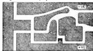
Fig. 3: An actual-size representation of the printed circuit board ( 1\frac{1}{8} in. x \frac{1}{4} in.).
